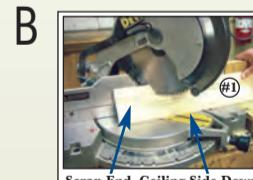
**B** How to cut piece #1: Place crown moulding (Figure 4, #1) ceiling side down in the mitre box. Set mitre box at 45° to the right and make cut.
